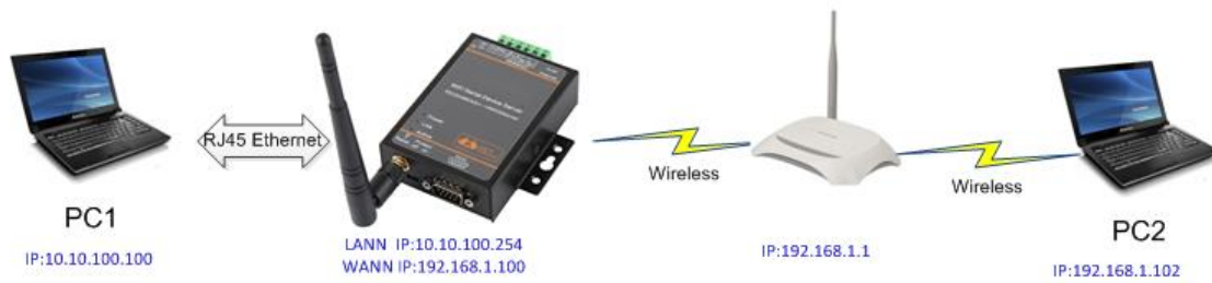
Figure 21. Ethernet Interface Function(Router)
